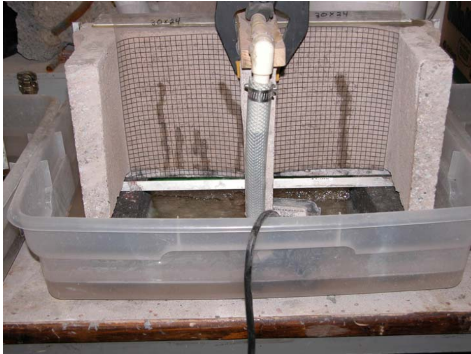
Figure X1.1: Example of tested specimen with pinholes on the inside of the front face shell
